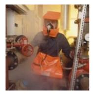
**Compressed Air Escape Set** – these are carried into the space by the worker, placed next to the work area, and only used once the gas monitor alarm goes off or if some other atmospheric hazard appears. They are only used for SHORT ESCAPE – approx 5- 15 minutes
