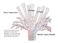
**Static Kernmantle** is rope constructed with its interior core (the kern) protected by a woven exterior sheath (mantle) designed to optimize strength, durability, and flexibility. The core fibres provide the tensile strength of the rope, while the sheath protects the core from abrasion during use. The name is derived from the German word *Kernmantel*, which means *core*[-and-]jacket.
