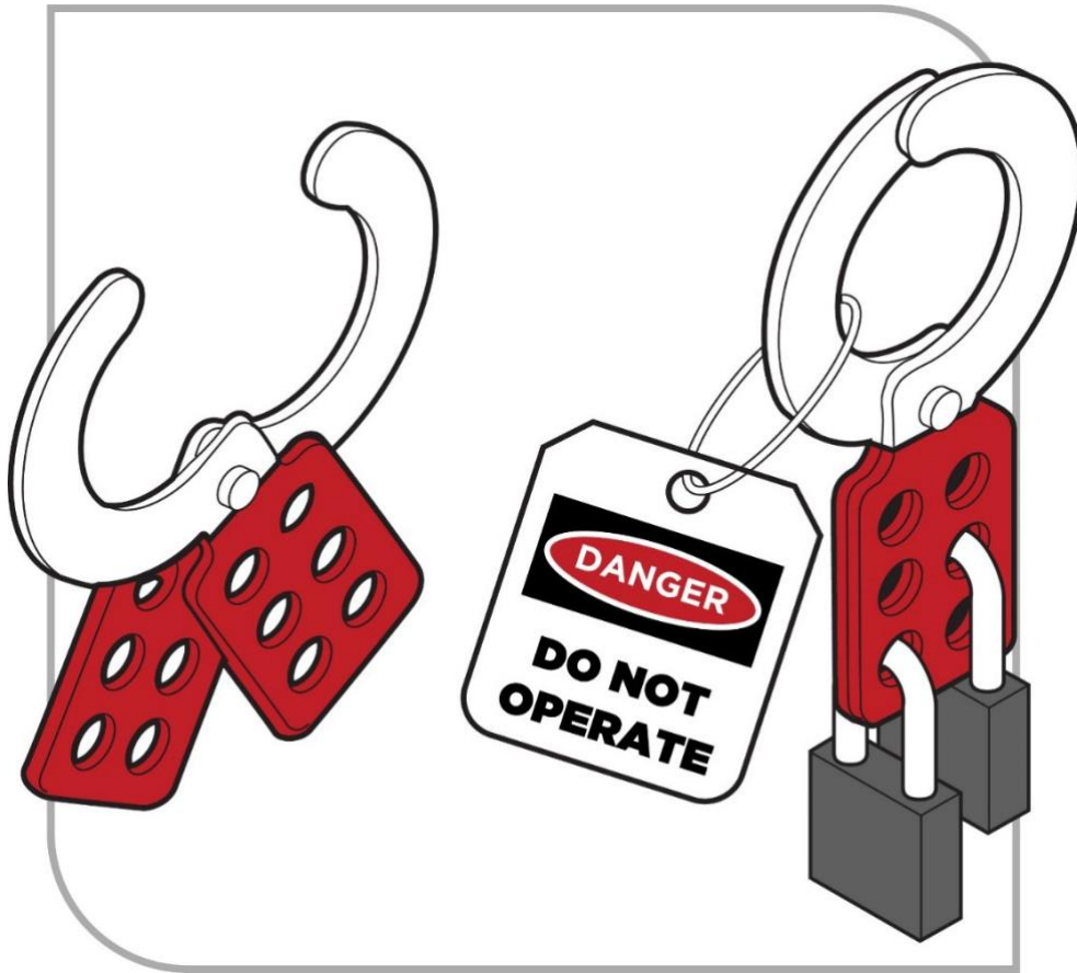
Figure 3 Example of tag and lockout with padlocks
