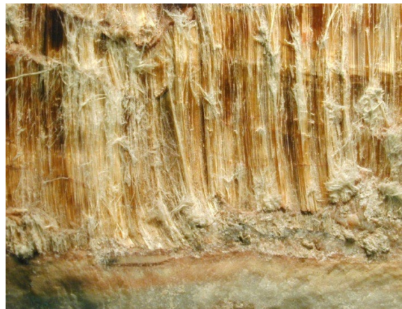
Amosite or 'Brown Asbestos'
